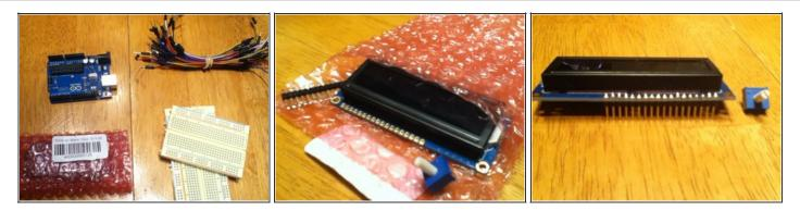
• We will start off by gathering all of the parts together. Then open the package. Inside, you will find the display, contrast pot, and header pins. Solder the header pins on the same side that I did.
